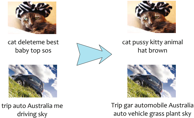
Figure 11.4. Examples of tag refinement. The left side of the figure shows the original tags while the right side shows the refined tags. The technique is able to remove irrelevant tags and add relevant tags to obtain better description of multimedia contents.
